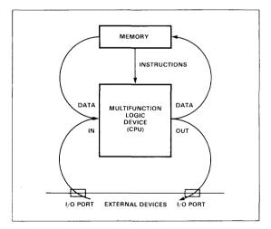
Fig. 2-2. Data and Instruction Paths in a Multifunction Logic Device
