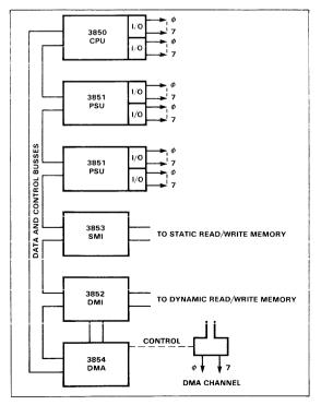
Fig. 2-5. F8 Microprocessor System Configurations
