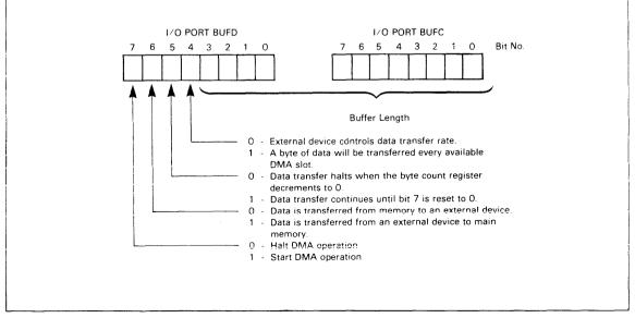
Fig. 8-4. How BUFC and BUFD are used to Control DMA Operations
