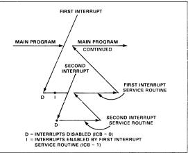
Fig. 8-2. Two Levels of Interrupt
