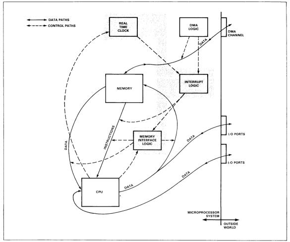
Fig. 2-11. Logical Functions of the 3853 SMI Device
