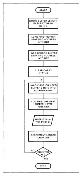
Fig. 3-2. Flowchart for Program to Add Two Multibyte Numbers and Output the Result
