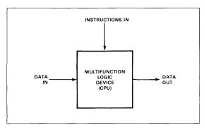
Fig. 2-1. Multifunction Logic Device
