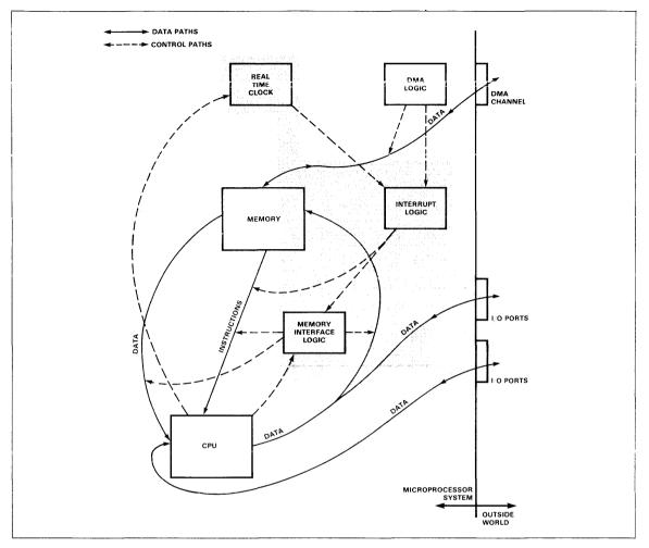
Fig. 2-9. Logical Functions of the 3851 PSU
