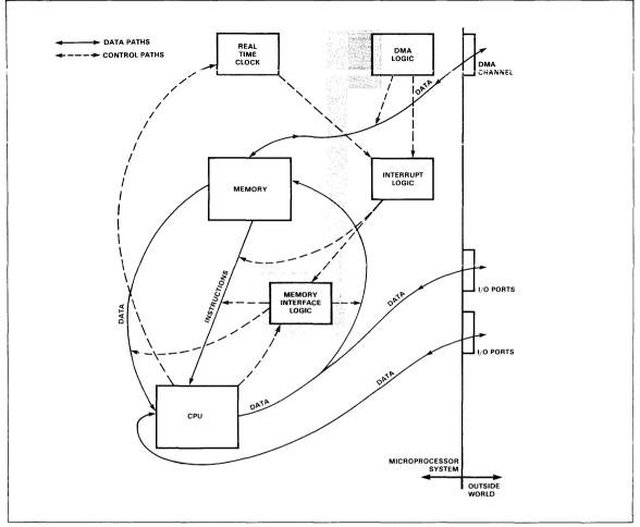
Fig. 2-10. Logical Functions of the 3852 DMI Device
